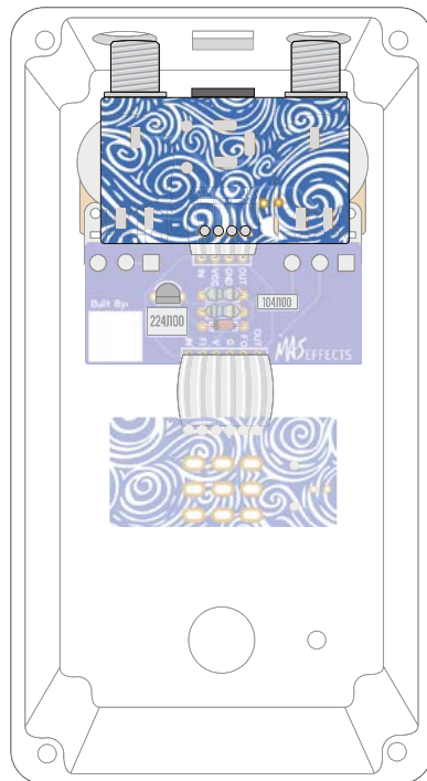
Solder PCB to Ribbon
