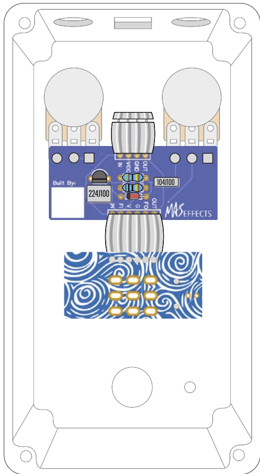
Solder main PCB to potentiometers.
